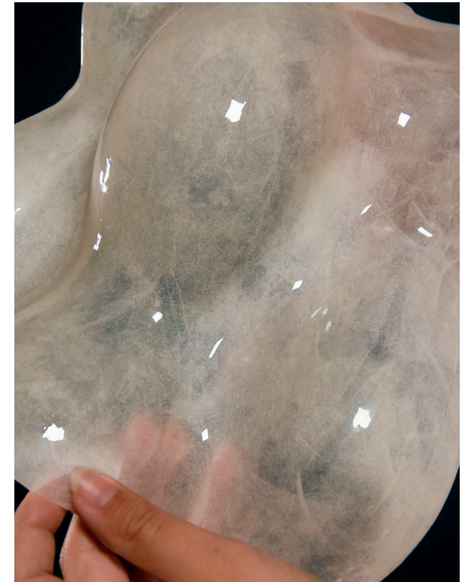
Molding sample, visible fibers, bio-based resin with glossy effect.
