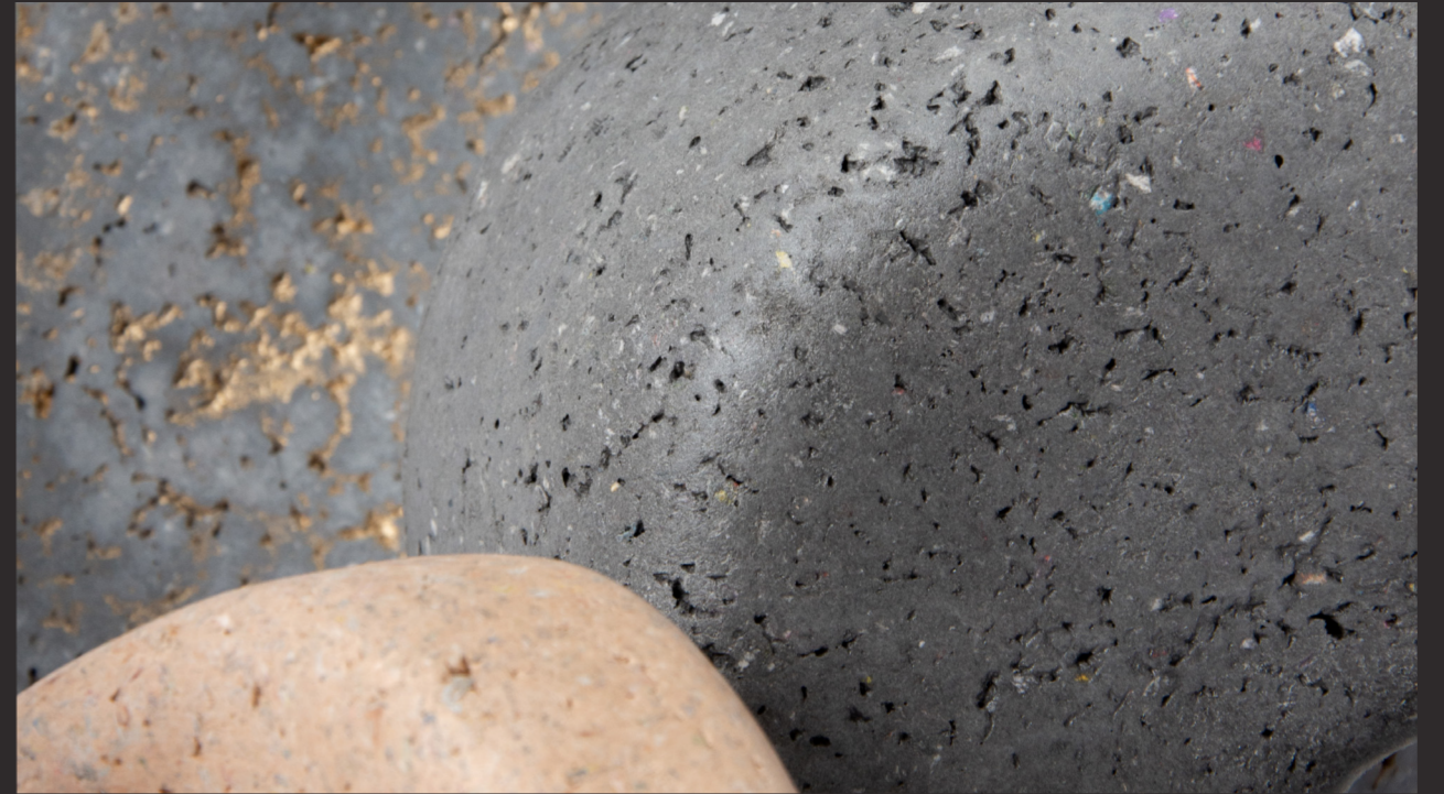
Matière Papier is an eco-responsible composite made from recycled cellulose. Cold-processed, this solution can be moulded or shaped and is intended for interior applications.
