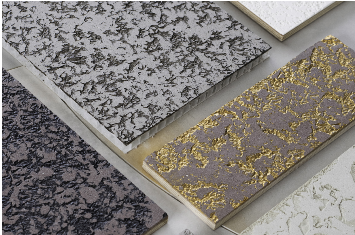
Sample, shaped render, forged, in thin layers.
